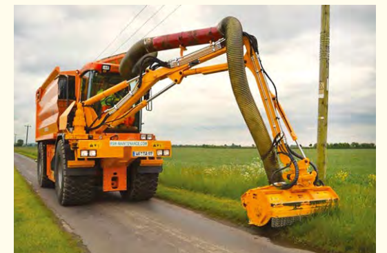
A tractor-mounted suction flail cutting verges in Lincolnshire, allowing simultaneous cut and collection of the grass, ready to be sent to an anaerobic digestion plant
